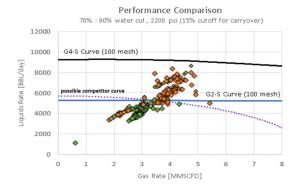
Overall, the competitor units on this trial captured less sand, less efficiently, while seeing lower overall liquid volumes. This reduction in flow rate may be due to higher back pressure across the competitor (non-Vapor Lock) spheres.
