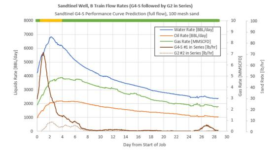
This trend shows the superior sand separation of the G4-S Maverick which handled nearly twice as much flow as either G2 Defender on the A Train. The G4-S captured almost all of the sand on the B Train, which saw 5,900 lb total. The downstream G2 Defender captured the remainder, and no sand was seen in the downstream 4-phase separator tank.
