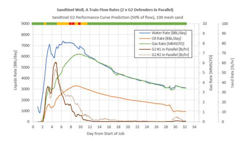
This trend clearly shows approximately even split of flow between the two G2 Defender Sandtinel units, with a high volume of sand captured on each one (11,600 lb total between the two of them). The yellow and red regions along the top show periods of high flow rate where the conditions were outside of Sandtinel's operating envelope. During these periods, lower than 95% efficiency would have been expected.
