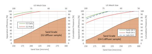
The efficiency as estimated in CFD simulations is shown below for the five selected operating conditions. G2 conditions are from the A Train and G4-S conditions are from the B Train.
