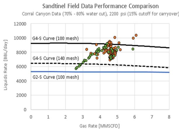
On this figure, the green dots indicate hourly measurements of flow rates where a minimum of 85% separation efficiency was seen in the upstream G4-S Maverick sand separator. Orange dots indicate hourly measurements where less than 85% efficiency was seen.
