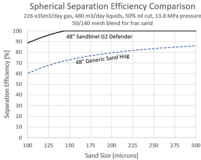
This condition is representative of Sandtinel's typical findings, which is that even at the conditions where generic spheres perform well (eg. at 200 microns and above in this chart) they rarely ever see better than 85% efficiency. Sandtinel's typical target for performance is a **minimum** of 95% separation efficiency, but in general Sandtinel spheres have the **highest efficiency which is mechanically possible without using filters**.
