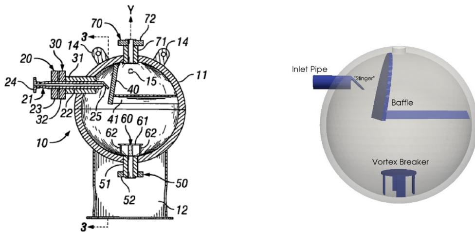
In CFD analysis of the Super Sand Hog, Sandtinel found that the main features for sand removal were a “stinger” on the inlet pipe and a slanted baffle which acts as a barrier to the flow. Fluid and sand are pushed down into the bottom of the vessel; the fluid circulates back up to the outlet pipe at the top, while some sand is retained in the lower hemisphere.
