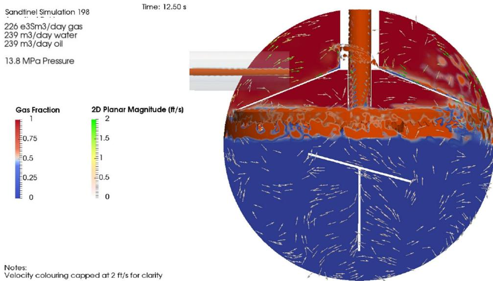
This CFD model allows Sandtinel to predict separation efficiency based on a wide range of criteria and to provide guidance on operational decisions about how to best use the equipment. Sandtinel’s typical criteria for performance targets a minimum of 95% separation efficiency, which has been proven to be achievable in basins all across North America.
