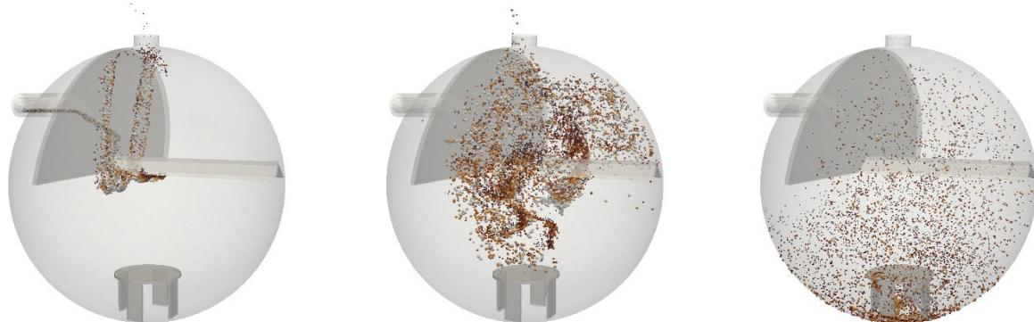
Heavier and larger sand is able to settle into the bottom of the Sand Hog, but a large fraction of the smaller sand is pulled straight up and out of the outlet pipe.
