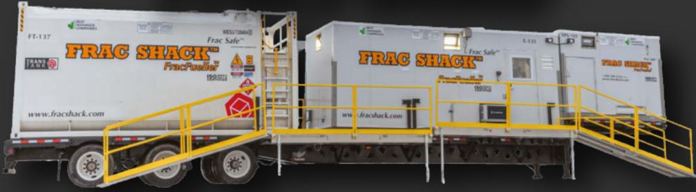
Fuel on the fly with no pressurized lines reduces spills, eliminates non-productive time, & removes workers from high risk, hazardous hot-zones. The diesel FracFueler™ operates up to 28 diesel lines using custom diesel flex-hose lines equipped with quick-dry connects.
